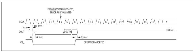
Figure 10. Aborted SPI Programming Operation (Invalid, Showing t<sub>CSDOZ</sub> and Internal Activity)
