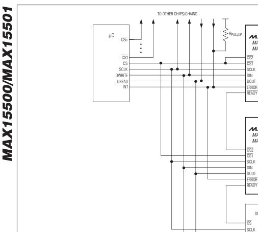
Figure 6. Daisy-Chain Terminating (Compatible with Standard SPI)
