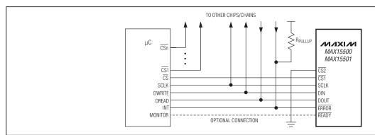
Figure 4. Alternate Single Connection (Compatible with Standard SPI)
