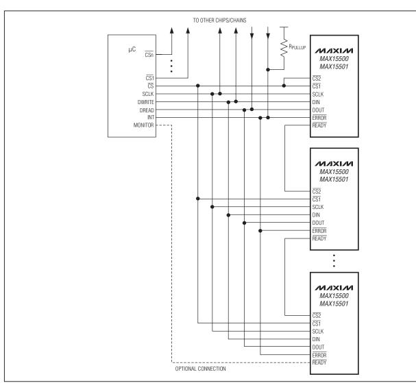
Figure 5. Daisy-Chain Connection (Compatible with Standard SPI)
