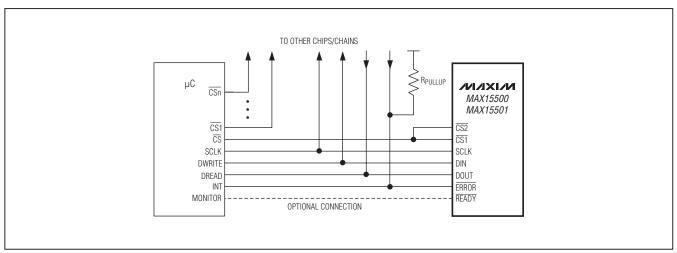
Figure 3. Single Connection (Compatible with Standard SPI)
