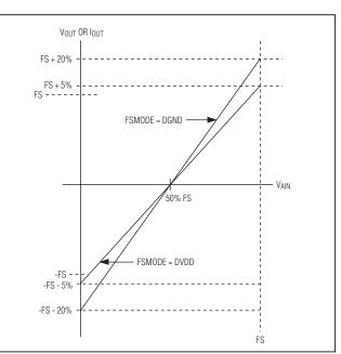
Figure 2. Bipolar Transfer Function
